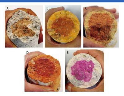
Concrete cores stained with curcumin solutions of 0.25% (A), 0.50% (B), 0.75% (C) and 1% (D) and with phenolphthalein solution 1% (E).
